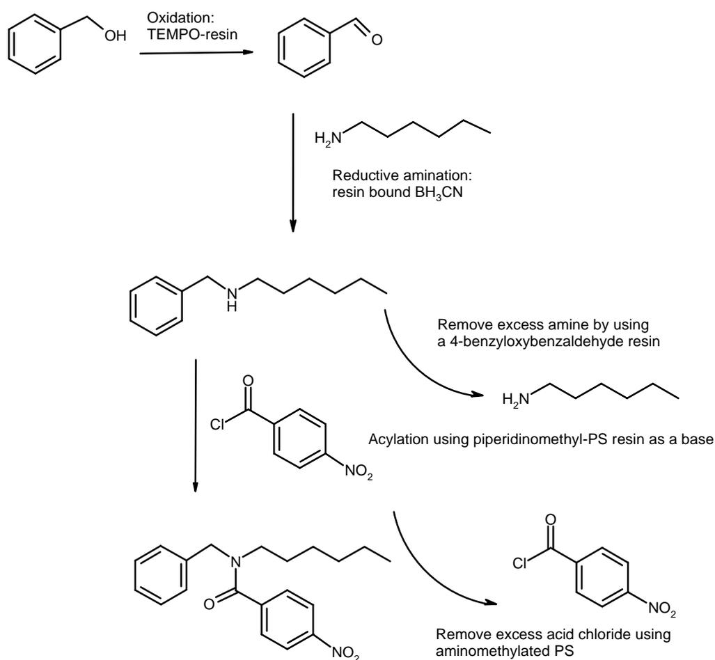
**Figure 7:** A simple reaction sequence with polymer supported reagents.
