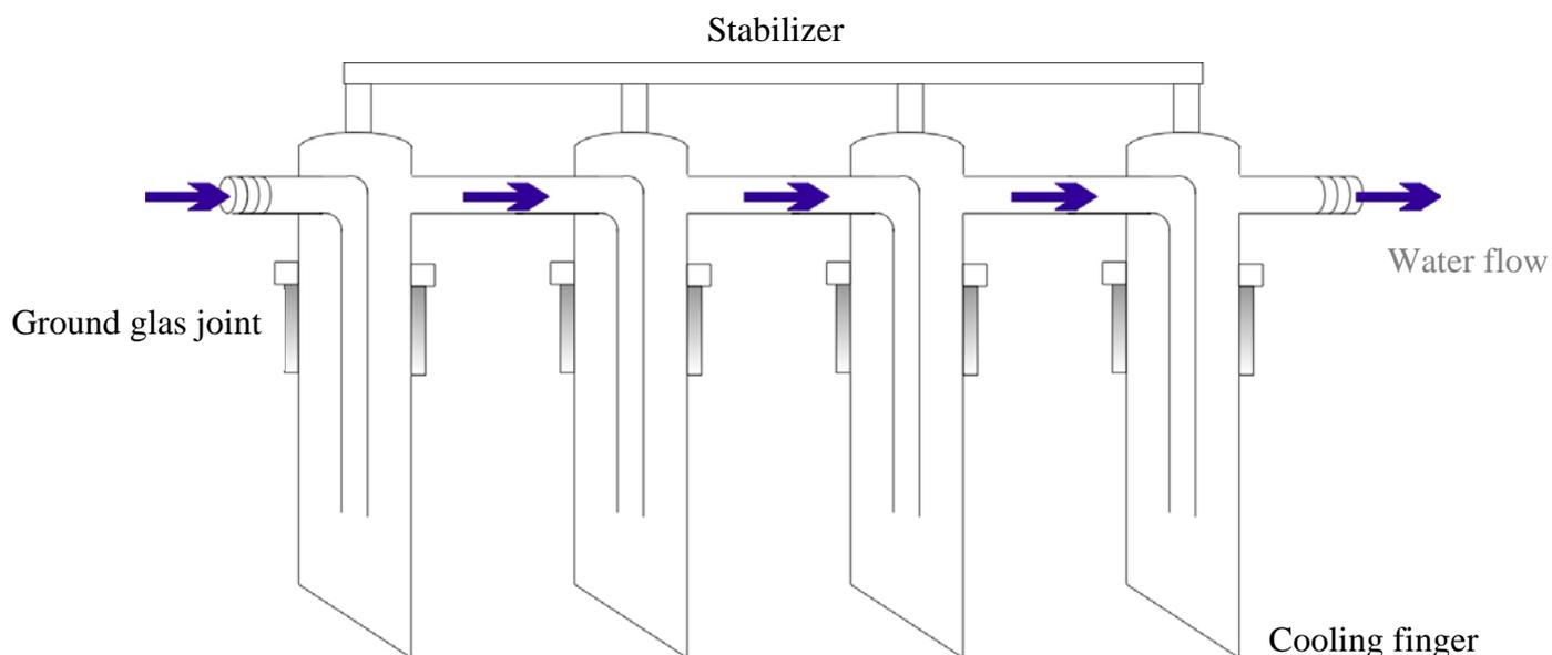
**Figure14.** Scheme of Cooling system
