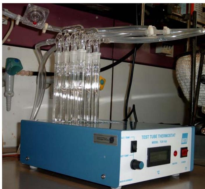
**Figure 13.** Parallel esterification using test tubes in a heating block
